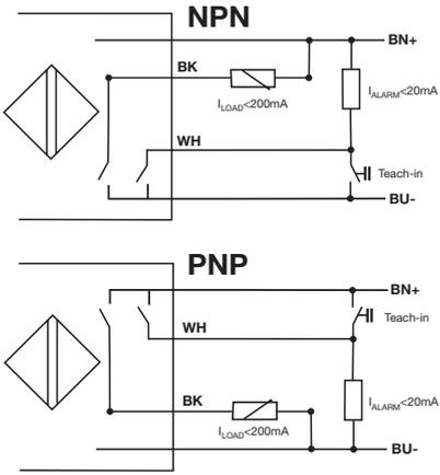
By means of the Teach-in wire, the functions described in the Teach-in Guide can be setup.
